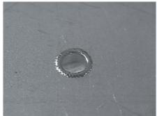
Figure 6 Laser weld repair of the inside diameter of an <sup>1</sup>/8-in. hole.
